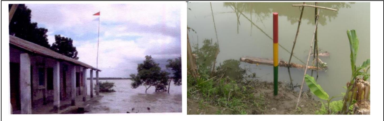
Figure: Hoisting of Danger Flag and Flood Pillar Showing Different Flood Level
